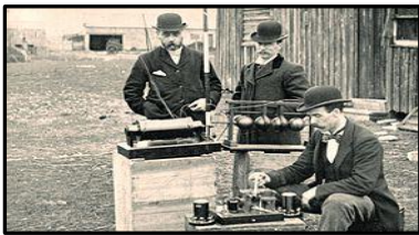
British Post Office engineers inspect Marconi's radio equipment during demonstration on Flat Holm Island, 13 May 1897. The transmitter is at centre, the coherer receiver below it, the pole supporting the wire antenna is visible at top
